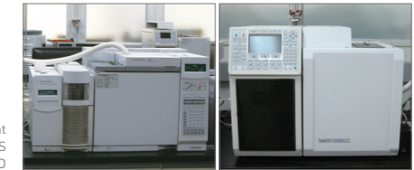
Main R&D Center test equipment TD/GC/MS SPME/GC/NPD
